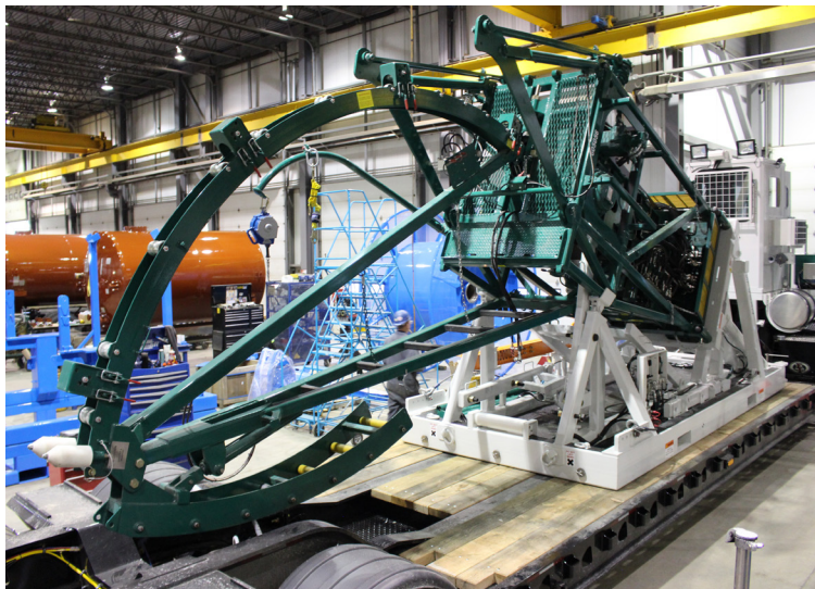
HR-6140 injector on hydraulic tilt frame; equipped with stabbing winch
