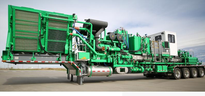
The Enerflow™ twin-engine fluid pump with 2,400 combined hp is designed to meet the growing demands of today's fluid pumping market. From coiled tubing support to standalone well servicing requirements including pump down, clean outs, reverse circulation, fluid swab-outs, well kill operations, pressure control, pressure testing, and reservoir stimulation, this twin fluid pump will exceed expectations.
