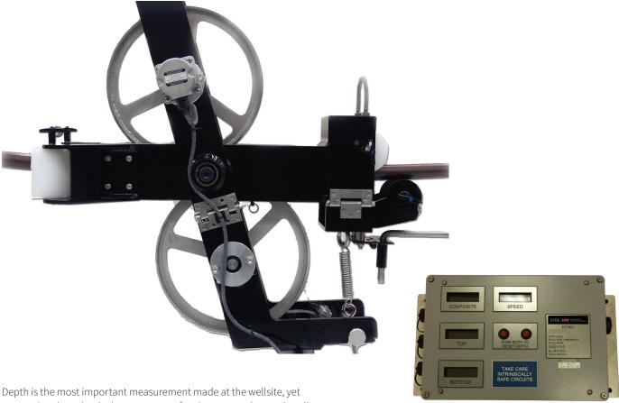
conventional mechanical counters are often inaccurate due to pipe slippage passed the single small-diameter friction wheel.
