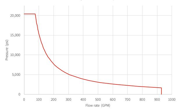
WS-1000-S Hydraulic Horsepower
