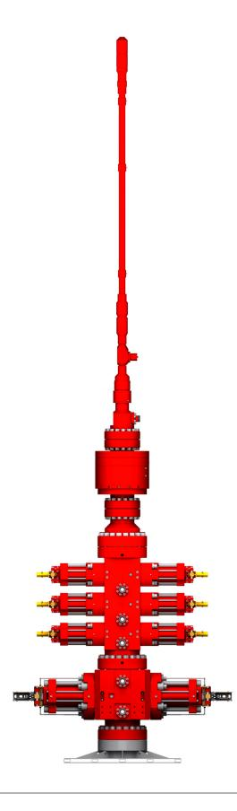
Our subsea products can help you save time and money during subsea well interventions. In this configuration we have both an ET series single safety head and an EIA series triple wireline BOP. The safety head is a blind shear ram that meets the requirements of NORSOK D002 for a safety head. The EIA triple BOP meets the requirements of ISO 13628-7 for a subsea well intervention BOP.
