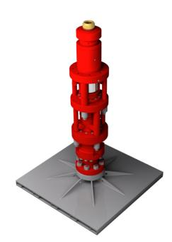
An industry first, our two-door stripper assemblies incorporate two independent packer elements that are compressed by independent pistons and hydraulic circuits. With doors on each packer element, this assembly setup allows easy access to change out elements and wear brass under pressure. This functionality allows quick element replacement with pipe stabbed, reducing NPT and safety risk.
