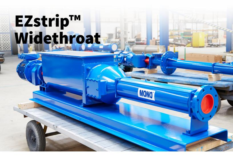
The EZstrip Widethroat pump is designed with a large auger inlet and screw conveyor. The screw conveyor extends to the compression area to help push the sludge cake into the cavities of the rotor and stator and provide consistent pumping.
