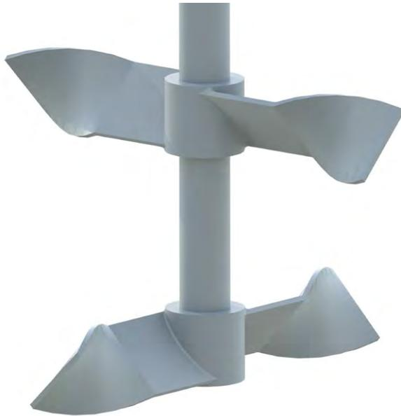
The JT-2 impeller is used for superior blending in transitional flow. High viscosity and non-Newtonian fluids make blending much more challenging. This impeller is used after conventional turbines have lost efficiency due to viscous effects and before the need for close clearance impellers.
