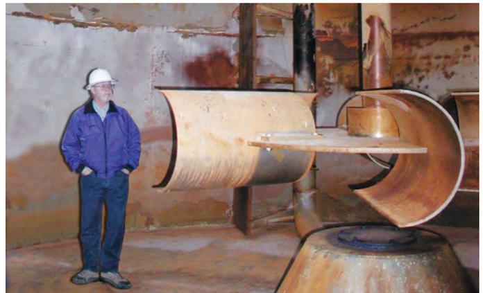
Chemineer agitators can be equipped with a large range of impeller styles and sizes
