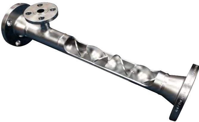
KM static mixers feature a patented helical mixing element which produces complete radial mixing and flow division for any combination of liquids, gases, or solids.
