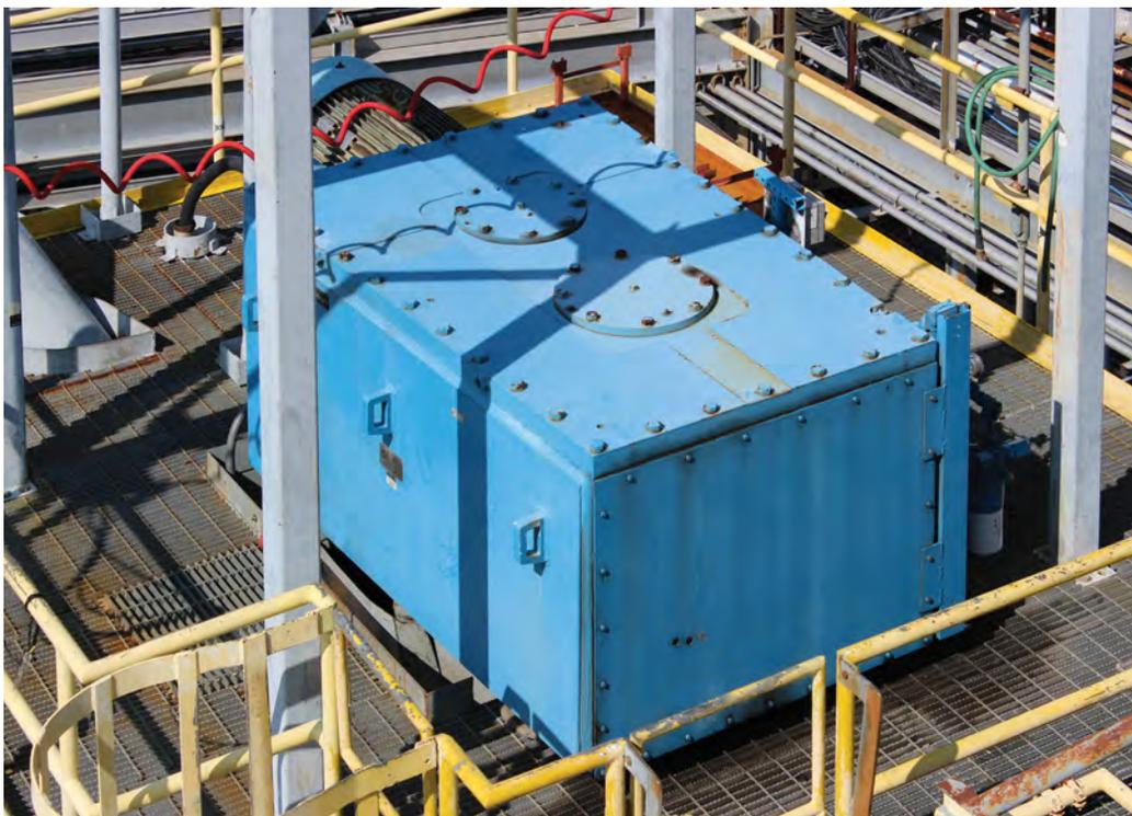
Installed Chemineer HT agitator
