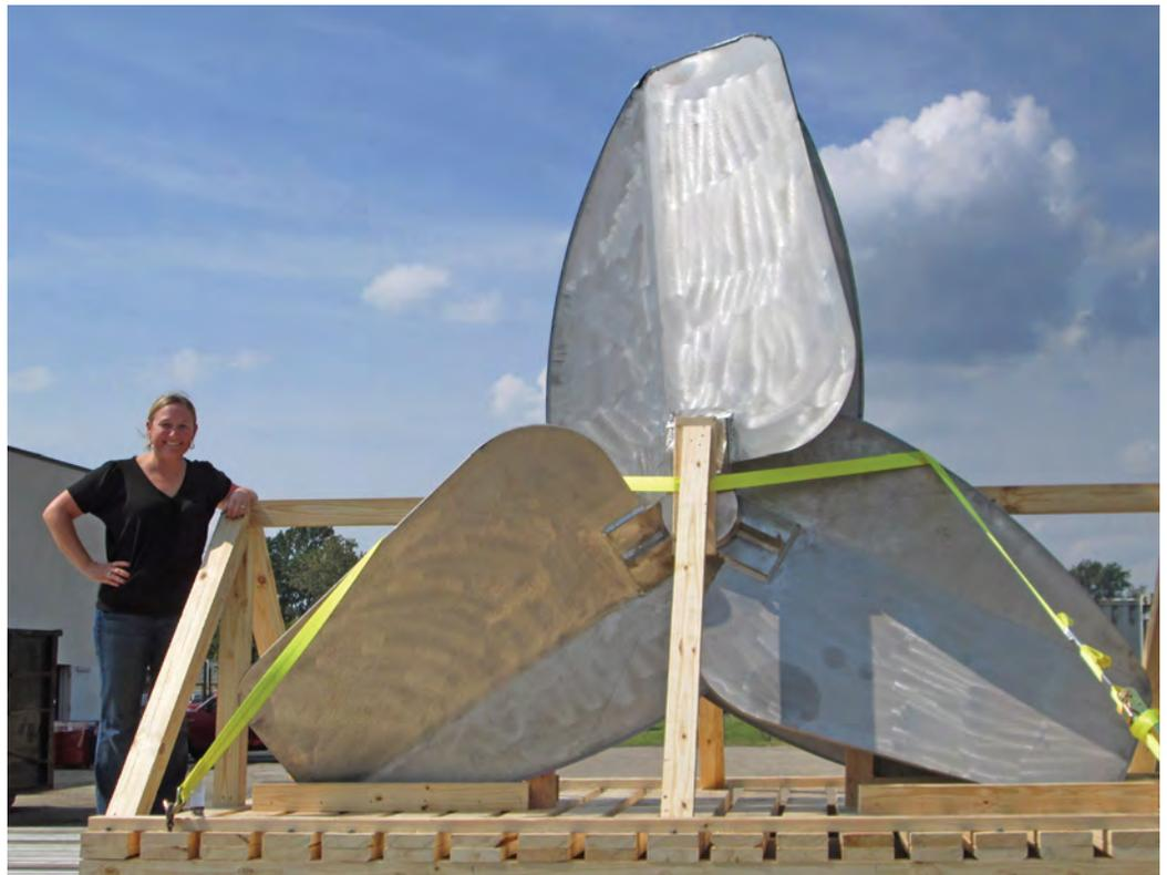
120" RL-3 impeller shipping to a facility in Florida to be used to prevent fibrous buildup in an application where ragging is a significant issue
