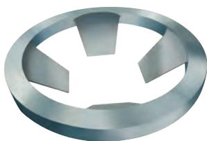
HEV high efficiency static mixers handle all turbulent flow mixing applications regardless of line size or shape. Mixing is accomplished by controlled vortex structures generated by the patented low profile tab geometry. This provides uniform blending while limiting mixer length to less than 1-1/2 pipe diameters. Complete mixing is achieved with pressure losses 75% less than conventional static mixers.
