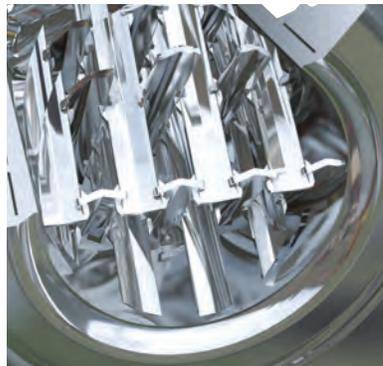
*Low viscosity additives are driven along the trough of each blade and abruptly sheared by strong cross-stream velocity gradients as they pass around the upstream surface*
