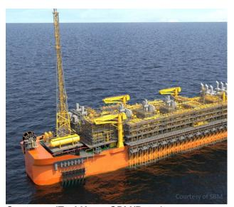
Customer/End User: SBM/Petrobras Solution: 276,800 BPD module consisting of coarse filters, UF, SRU feed pumps, SRU, RO booster pump, SWRO, CIP, chemical dosing skid, deaerator, and SW booster pumps.
