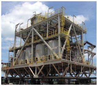
Customer/End User: Modec/Tullow Oil Solution: 232,000 BPD modules consisting of coarse filters, multimedia and guard filters, deaerator, and SRU. NOV provided lifecycle services including digitalization with NOV PIM.
