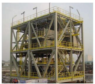
Customer/End User: Modec/Petrobras Solution: 120,000 BPD module consisting of coarse filters, cartridge filters, SRU, and deaerator. Project was delivered in 38 weeks.
