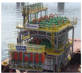
Customer/End User: Petrobras Solution: 220,000 BPD skid-based solution consisting of coarse filters, cartridge filters, SRU, deaerator (loose), and injection pumps.
