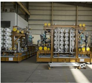
Customer/End User: Grupo Avanzia/Hockhi Solution: 300 m<sup>3</sup>/h SW + 300 m<sup>3</sup>/h PW. Coarse filters, multimedia filters, deaerator, and SRU.
