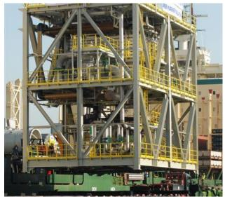
**Customer/End User:** Modec/Petrobras **Solution:** 138,000 BPD modules consisting of coarse filters, cartridge filters, SRU, and deaerator (loose)
