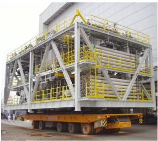
**Customer/End User:** Modec/Petrobras **Solution:** 31,400 BPD module consisting of coarse filters, multimedia and guard filters, deaerator, and SRU.
