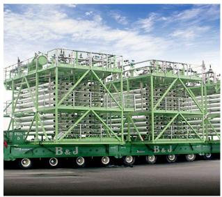
Customer/End User: Petrobras/Triton Energy Solution: 135,000 BPD skid-based solution consisting of cartridge filters, and SRU.
