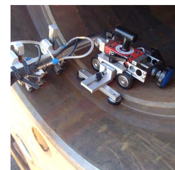
Riser main tube flange pocket inspection tool
