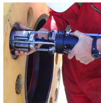
Riser auxiliary line pulse echo UT inspection tool
