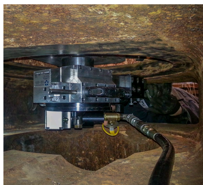
Blowout preventer bore seal seat machining tool
