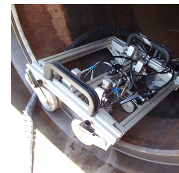
Riser main tube phased array UT inspection tool
