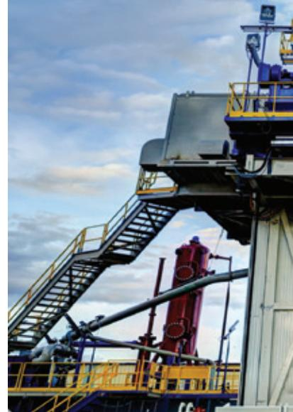
Available in two distinct and powerful classes — 1,500-horsepower, 350-ton and 2,000-horsepower, 500-ton — the European Rig is the complete drilling package for drilling within the European Union. European 1500 equipment suite is shown; equipment may vary based on rig horsepower options.
