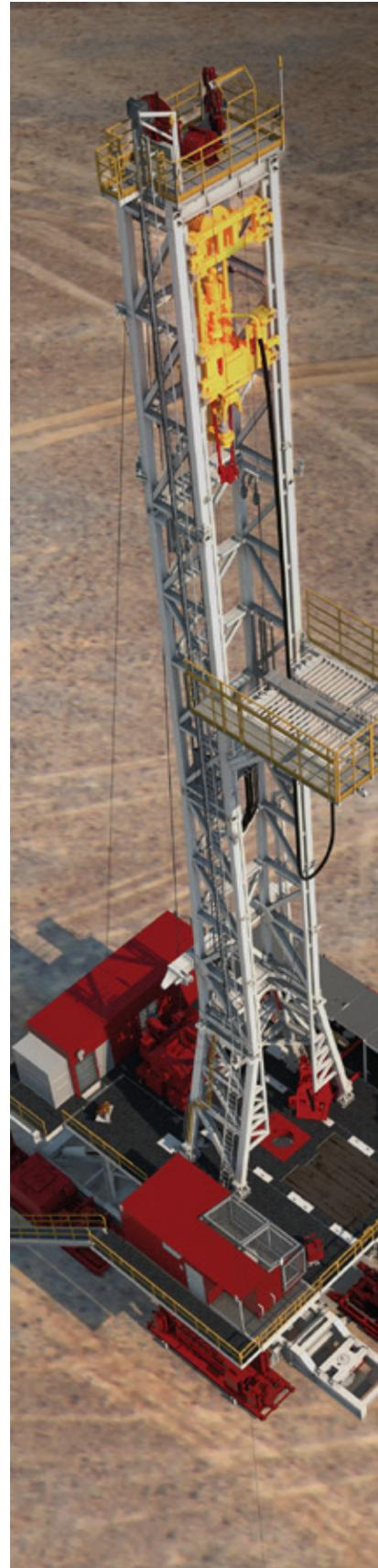
Our new Ideal 2000 land rig is a fully integrated, configurable land rig designed to meet the needs of today's increasingly complex drilling conditions. The NOVOS™-enabled rig has 2,000 horsepower and increased setback capacity, allowing it to drill deeper wells and longer laterals.
