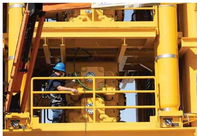
**20K Subsea BOP packaged where equipment has maintenance access to line up with platform access in the moonpool.**
