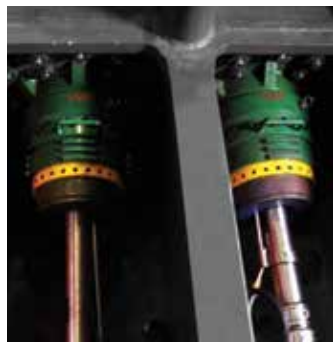
Blak-JAK Liner Retention System mounted in a pump
