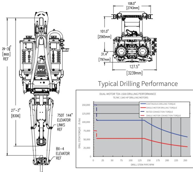
The TDX-1500 is the latest incarnation of NOV's successful TDX Top Drive product offering. Leveraging from the success of the TDX-1000 and TDX-1250 this unit is designed around the same key design principles. Safety, reliability, redundancy and modularity are at the core of the TDX-1500 design. The TDX-1500's compact design offers an industry-leading hoisting capacity of 1500t and handles the extreme demands required by the latest generation of ultra-deepwater and 20K ready drilling rigs.
