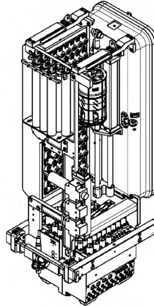
LMRP Module removed from pod frame
