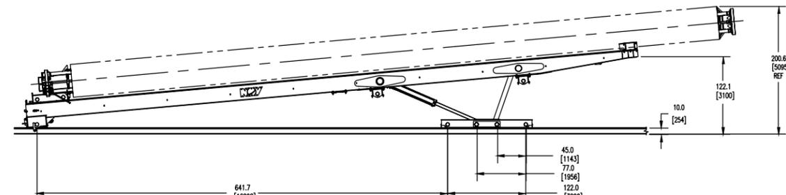
The Riser Handling System (RHS) uses a hydraulically powered trolley-on-a-trolley to accomplish two tasks. (1) Transporting horizontal riser joints from the riser deck to the well center. (2) Safely tailing the riser section while it is hoisted by the drawworks from a horizontal to vertical position. The system can accommodate various requirements of riser length, diameter, and riser spider/gimbal height.
