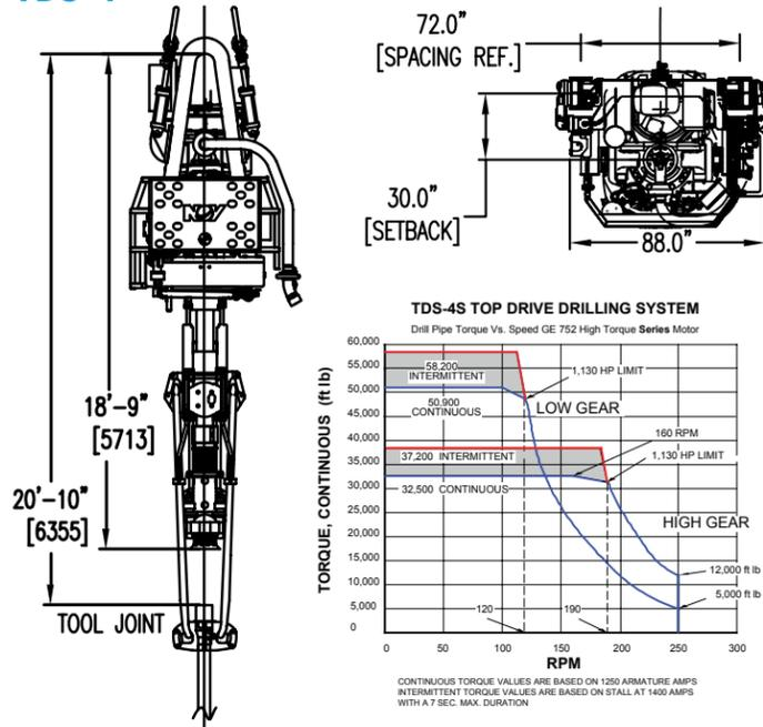
The TDS-4S is our prime large bore DC top drive. It has built its reputation by performing well in the heavy drilling environments found offshore. This 750 ton top drive has been in service and operation since 1988 and over 350 units have been in service since that time. Although considered a mature product, its high demand in the top drive market today is a tribute to its robust and reliable reputation built on years of drilling experience.
