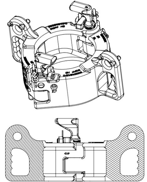
The SJX single joint elevator is designed for running single joints of tubing and casing from V-door to well center. It is double hinged for use with the CRT Casing Running Tool, or any other stabberless operation. Ergonomically designed handles with cast on stop pins prevent the lifting sling shackles from pinching hands. Suitable for loads up to 5 sTon / 4.5 Tonne.
