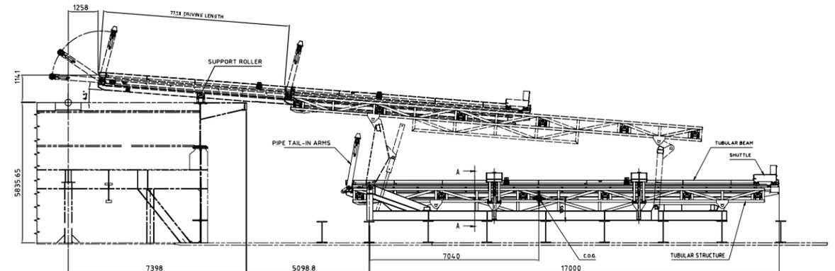
The Tubular Shuttle Machine (TS) is designed to transfer tubulars between the pipe-deck and the drill-floor. Tubulars can be removed from or landed onto the tubular beam using the elevator in combination with the front mounted Pipe Tail-in Arm. The design of the machine is basically very simple and utilizes tried and tested solutions. The design philosophy is intended to achieve minimum complexity, provide safe and reliable operation, and simplify maintenance requirements. It includes a modular
