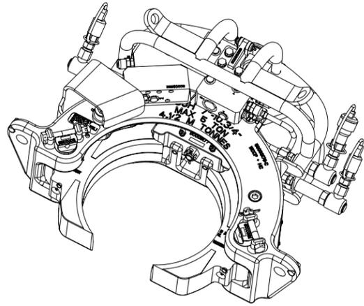
The SJH horizontal pick up elevator is designed to pick up tubulars lying flat on a surface without having to lift the tubulars prior to closing the elevator. The elevator is capable of lifting drill pipe, recessed/zip lift drill collars and casing. It will handle single joints of pipe straight from cantilever to off-line stand building systems.
