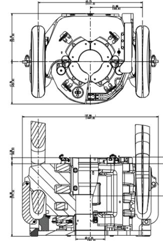
Construction of deepwater and ultra-deepwater drilling rigs created demand for equipment with a greater capacity. The BX9 has a rating of 750-1,250 sTon for 18° shoulder, 750-1,500 sTon for 90° (square) shoulder and 1,250-1,500 sTon for riser handling and 45° shouldered couplings.
