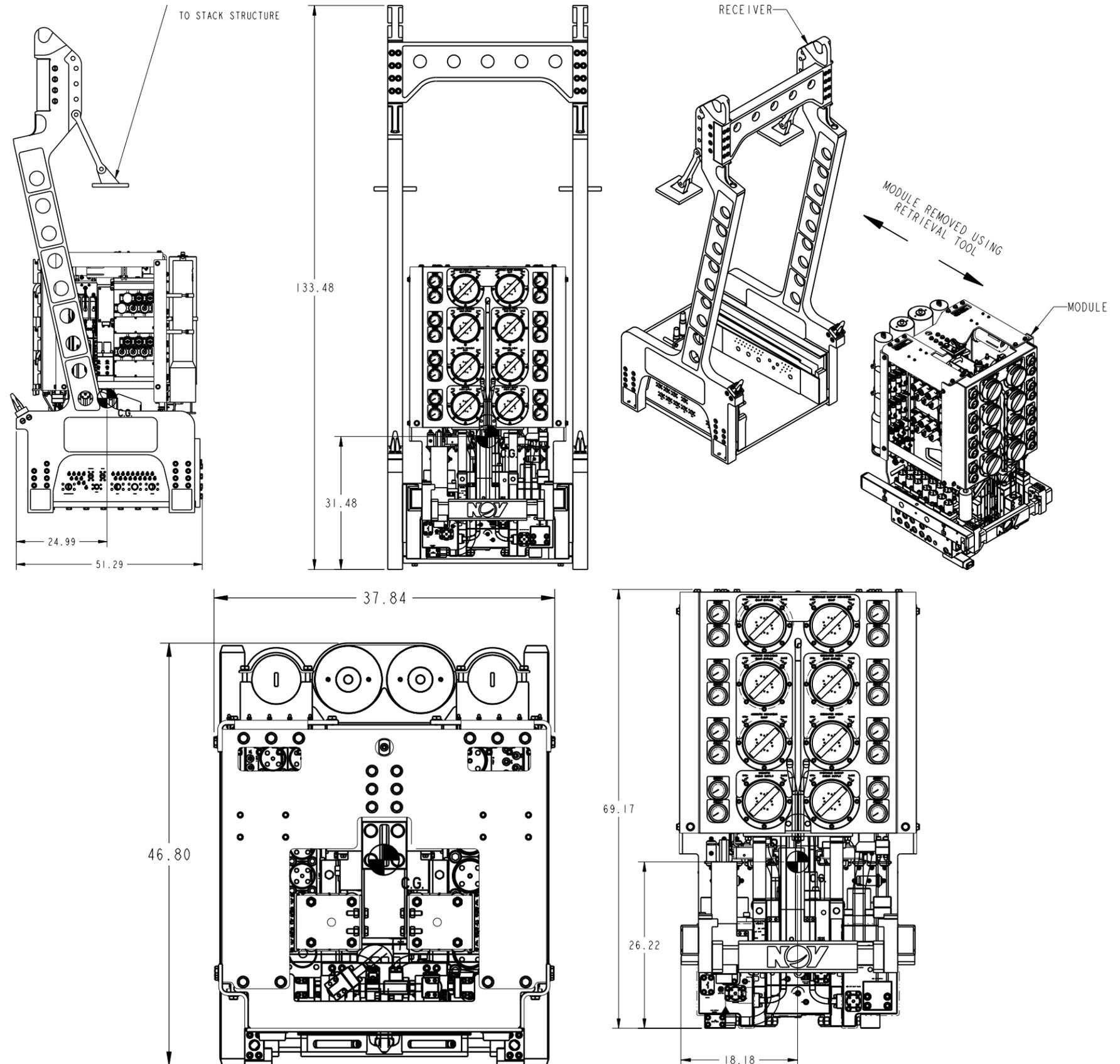
Today's designed operating environment for stack mounted accumulators is challenging. Design criteria include 12,000 ft water depths, temperatures as low as 32°F with surface temperatures of 120°F, rapid discharge (adiabatic), as well as higher minimum system pressures. All of these things add up to a large number of bottles on a lower BOP stack. It is not uncommon to see as many as 126 accumulator bottles on a
