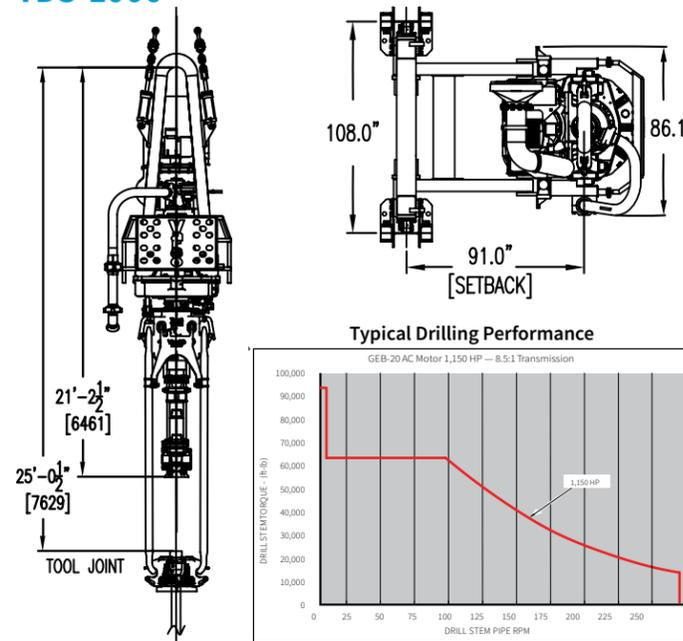
Developed for use in deep drilling applications, the TDS-1000 provides an intermittent torque output of 96,000 ft-lbs to make and break even the highest torque connections. Because of the broad speed and torque range provided by the AC motor, this performance is obtained using a single-speed gear box. The TDS-1000 Top Drive is driven by a Variable Frequency Drive (VFD) control system for a greater range of torque and speed performance.
