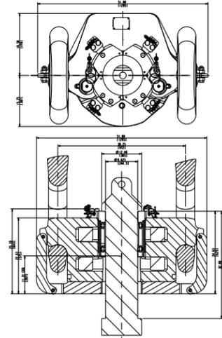
Construction of deepwater and ultra-deepwater drilling rigs created demand for equipment with a greater capacity. The SBX is a manual operated single door solid body elevator. It has a rating of 1,250 short tons for riser handling with square shouldered couplings/45° tool joints.
