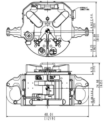
The BXS allows a safe way to run a small upset and special clearance tubulars with the new BXS elevator. This tool enables rigs to handle flush or near flush tubulars without manual intervention. The BXS provides reliable operation and is suitable for use with the FMS 275 Flush Mounted Slip.
