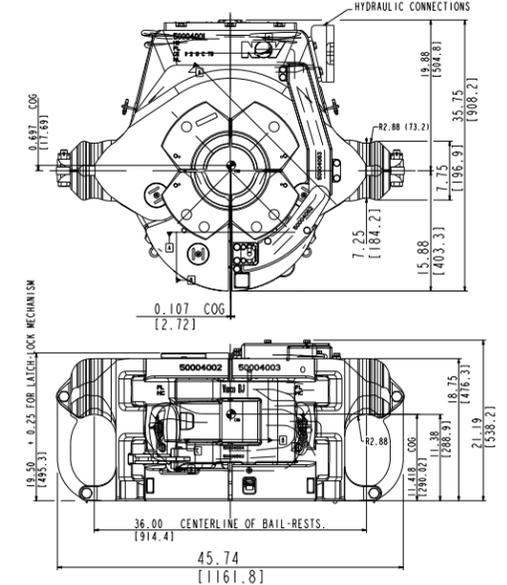
The BX 3, 4, and 5 elevators improve both rig safety and efficiency. Since the introduction of the BX 1 and 2 elevators in 1996, our engineers have continuously strived to improve the operations reliability and safety of its design, resulting in the present BX 3, 4, and 5 design.
