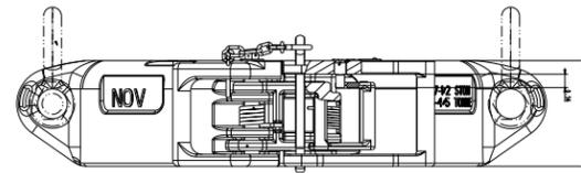
SJL and SPL single-joint, center-latch elevators are designed to replace unsafe rope slings for hoisting collar-type pipe into position. The SJL 90° elevator enables the crew to handle pipe properly, help avoid damage to pipe threads and reduce the chances of accident or injury. The SPL elevator is the same as the SJL elevator except that the SPL elevator is designed for use on tapered pipe, conforming to API specifications for extreme line casing.
