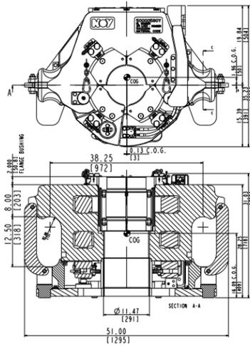
Construction of deepwater and ultra-deepwater drilling rigs created demand for equipment with a greater capacity. The BX7 has a rating of 1,000 short tons for drill pipe and landing strings, and 1,250 short tons for riser handling and square shouldered couplings.
