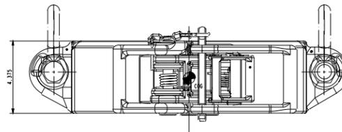
SJL and SPL single-joint, center-latch elevators are designed to replace unsafe rope slings for hoisting collar-type pipe into position. The SJL 90° elevator enables the crew to handle pipe properly, help avoid damage to pipe threads and reduce the chances of accident or injury. The SPL elevator is the same as the SJL elevator except that the SPL elevator is designed for use on tapered pipe, conforming to API specifications for extreme line casing.
