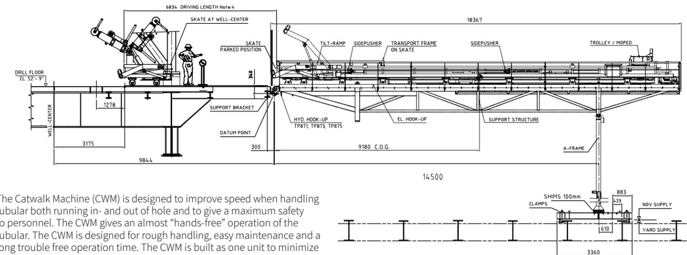
The Catwalk Machine (CWM) is designed to improve speed when handling tubular both running in- and out of hole and to give a maximum safety to personnel. The CWM gives an almost "hands-free" operation of the tubular. The CWM is designed for rough handling, easy maintenance and a long trouble free operation time. The CWM is built as one unit to minimize installation costs on the rig.
