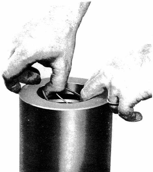
Figure 3 Place edge of Ring opposite the split into the lower groove and spread from center toward ends. Be sure beveled side of ring matches beveled groove side.
