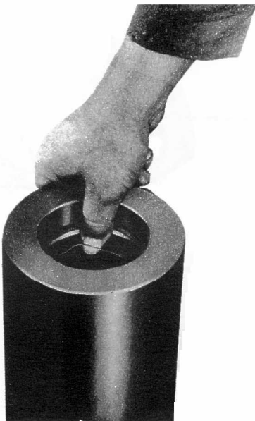
Figure 7 Insert one edge in groove. Then insert the opposite edge and press down until entire ring is in place.
