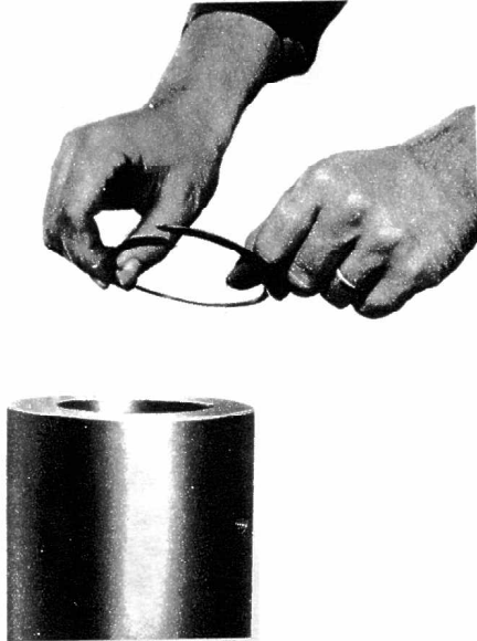
Figure 1 Hold Non-Extrusion Ring between thumbs and forefingers as shown.
