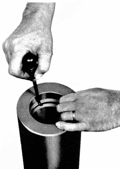
Seal Assembly Removal
