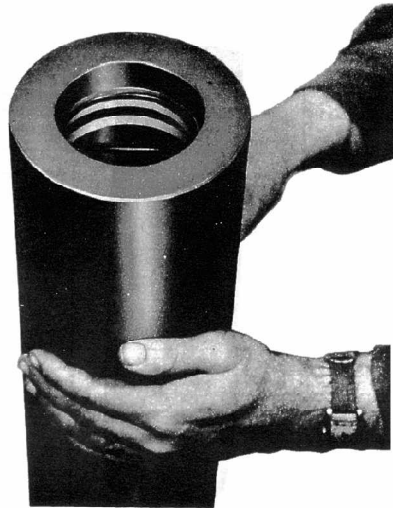
Figure 11 Insert O-Rings between Seal Protection Rings in each groove.
