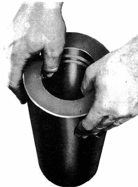
Figure 4 Using Thumbs, press Ring into groove until ends match up and ring is firmly seated in groove.
