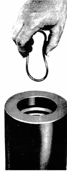
Figure 10 Bend O-Ring as shown to insert into groove.
