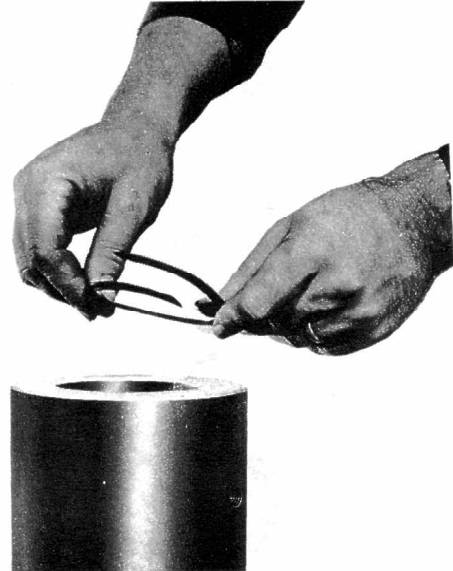
Figure 2 Overlap ends until diameter is small enough to fit inside body.
