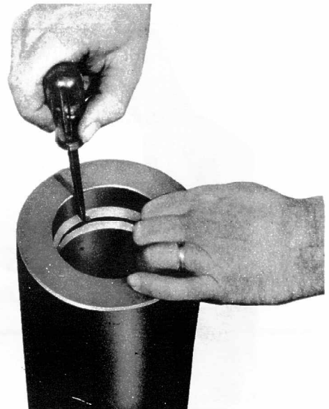
Figure 8 Use Seal Protector Ring installation tool to straighten and flatten ring by pressing against ring as shown.
