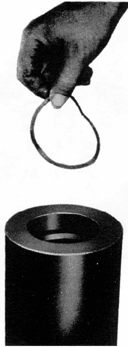
Figure 6 Bend the Ring until it is small enough to allow entry into bore.
