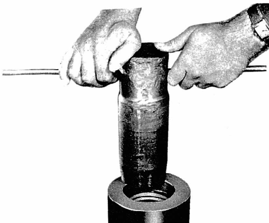
Figure 15 Insert the setting tool as shown. Use any convenient rod or bar to hold the tool.
