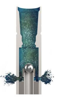
Pump pressure forces the piston valve down, opening the ports to the annulus and closing off flow through sensitive BHA components.
