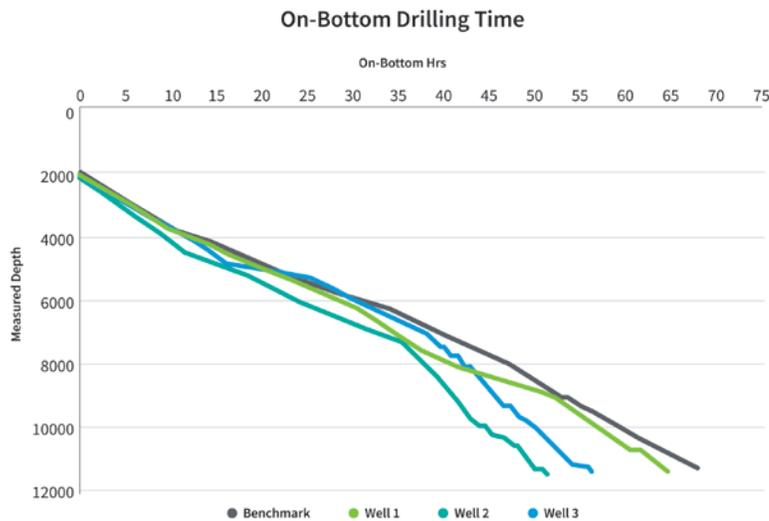
The KAIZEN system was assessed over a three-well span against a benchmark. On the first well, the customer held RPM static. On the second and third wells, the KAIZEN system was given a window in which to perform optimization functions. An ROP improvement of 61% and 39%, respectively, was observed in Wells 2 and 3 versus the benchmark. The customer allowed the largest parameter window for optimization in Well 2, and therefore the highest performance gains were achieved in that well.
