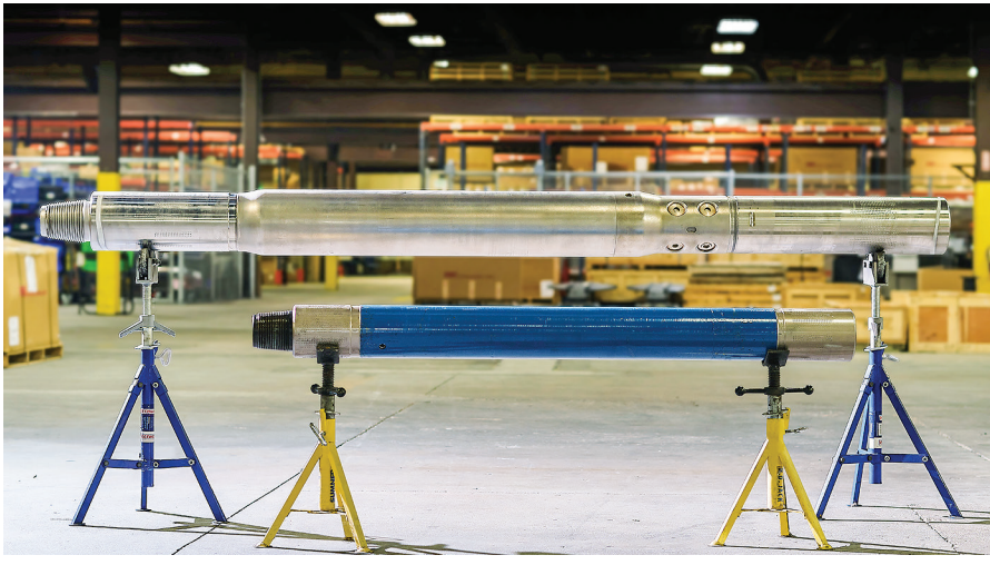
Fig. 2. BlackStream measurement tools for distributed sensor placement along the drill string.
