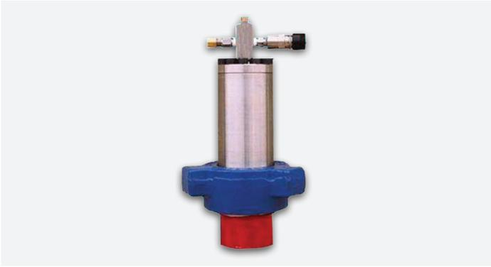
The 4:1 pressure deboosters are designed to reduce line pressure by a ratio of 4:1, exposing the operator at the panel  $\frac{1}{4}$  of the actual pressure that is seen at the manifold. Gauges are calibrated at  $\frac{1}{4}$  of the line pressure to reflect actual pressures.
