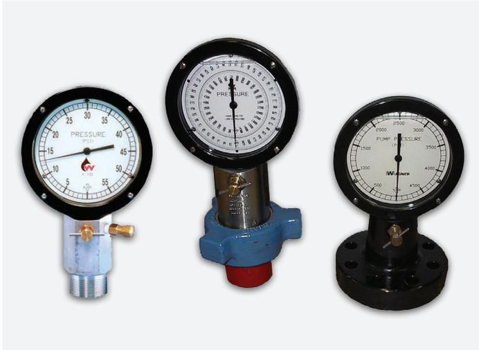
The standpipe pressure gauges are offered with a variety of connections, including 2" male npt, hammer union type, and flanged type. These gauges integrate a 6" inverted gauge with a heavy-duty housing and include a check valve and damper assembly incorporated into housing. These gauges are ideal for use on pumps, pump trucks, standpipe, choke manifolds, and pipeline pressure applications.
