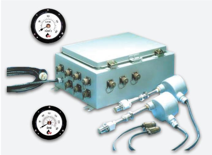
The proximity detection system eliminates the need for belt-driven generators on RPM and SPM systems. The system uses reliable and durable proximity sensors that are permanently mounted on the mud pump for the SPM and near the rotary table for the RPM. The signal received from the sensor is processed into an output signal in the form of a pulse signal or analog signal for operation of electric meters, digital pump stroke counters, recorders, etc.
