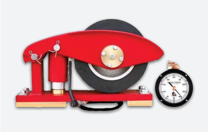
The rotary torque system-chain is designed to help the driller during coring, milling, and reaming operations. The system also helps avoid twist-offs and increases bit life by showing the driller when the drill string is torquing to unsafe levels.
