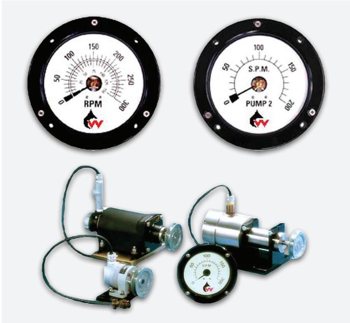
Tachometer generator systems are offered in both RPM and SPM versions. Both the RPM and SPM systems include a generator with mounting base, pulley, and v-belt with clip, cable assembly with connectors and j-box, meter assembly, and bracket to mount meter (box mount version only).
