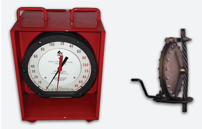
The deflection (clipper) type weight indicator is ideal for use with small drilling and work over rigs. The unit comes complete with 12" indicator with complete dial set, heavy-duty steel box for mounting, 25-foot hose, and deflection type sensor with c-clamp. Unit is ready to use out of the box and can be moved from rig-to-rig with ease.
