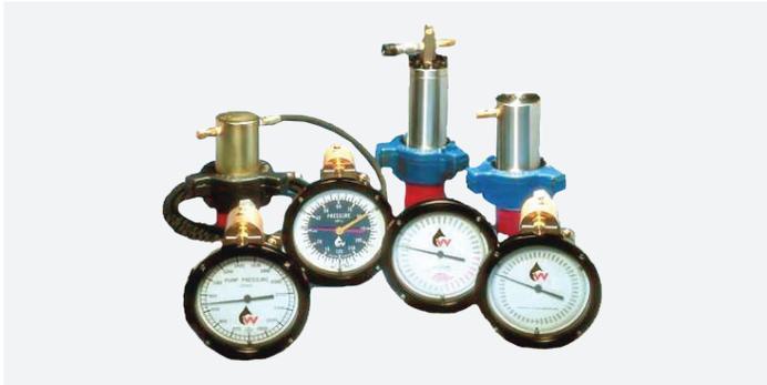
The pressure systems are designed to provide a quick, accurate check of pressure. The systems are available in both single pointer and dual pointer (compound) versions. Both types come complete with 6" liquid filled gauge, bracket to mount gauge (on box mount version only), hose assembly, sensor assembly (diaphragm protector, 1:1 piston isolator, or de booster), and recharge kit consisting of hand pump and (1) quart of instrument fluid.
