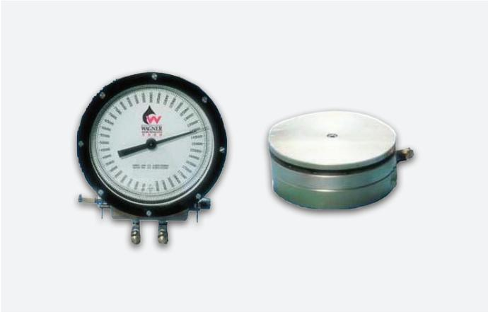
The hydraulic tank weight indicator system eliminates the guesswork when blending wet or dry material, providing extremely accurate load measurement for bulk tanks and hoppers. The system consists of gauge, bracket to mount gauge, hose assembly with disconnect set, load cell, and recharge kit consisting of hand pump, and (1) quart of instrument fluid.
