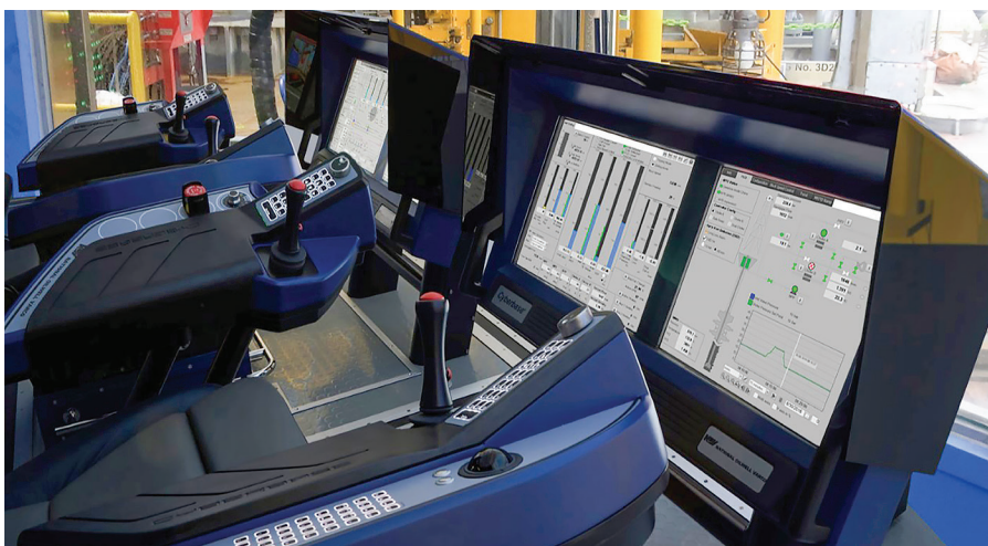
Fig. 1. From a single integrated screen, the driller is now in full control of the MPD and drilling operations, but with a lighter workload.
