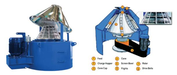
The VORTEX Dryer reduces and recovers base fluid from a variety of feed slurries. In drilling operations, shale shakers can discard drilled cuttings that are up to 20% oil by weight. Treatment with the VORTEX Dryer has proven to reduce this oil content dramatically, in some cases below 2%.
