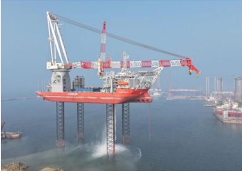
In the North Sea, Cadeler A/S took delivery of the Wind Peak, its first WTIV based on our NG-20000X self-propelled wind turbine installation jack-up vessel design. The vessel, which includes a heavy-lift crane with a capacity of more than 2,600 tons at 46 m (151 ft), can install seven complete 15-MW turbine sets per load or five sets of 20+ MW turbines. The early success of this design prompted Cadeler to order another NG-20000X vessel—the fifth NG-20000X order globally.
