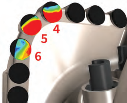
Comparison of shear stress across polycrystalline diamond compact (PDC) faces for conventional and HydroShear nozzles.
